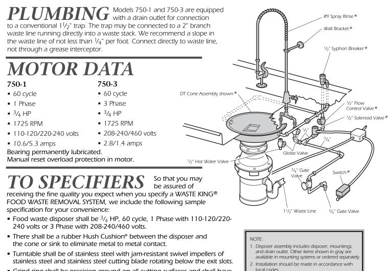
Grind ring shall be precision ground on all cutting surfaces and shall have non-wearing, size controlled exit slots.
