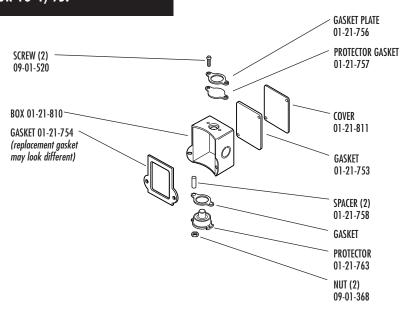
NEW STYLE BOX MAY BE USED IF REPLACING ABOVE ASSEMBLY.
