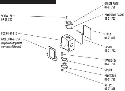
NEW STYLE BOX MAY BE USED IF REPLACING ABOVE ASSEMBLY.
